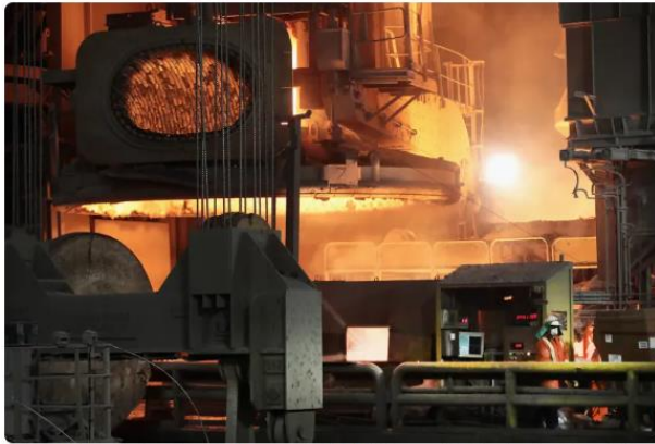
Workers monitor steel being melted at 3,000 degrees Fahrenheit (1,649 degrees Celsius) in an electric arc furnace (EAF) at the NLMK Indiana steel mill in Portage, Indiana, on March 15, 2018 [Scott Olson/Getty Images/AFP]
